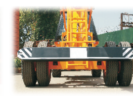
6 GROUND CLEARANCE High ground clearance of 400mm for easier rough terrain operation.
