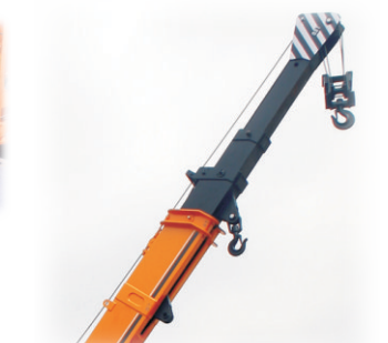
8 SLOTTED BOOM For easier load positioning
