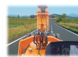
4 INCREASED VISIBILITY Bigger size front windscreen and re-routing of hoses provide much better front visibility.
